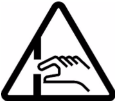
Warning sign for potential point of injury
