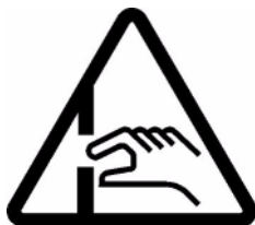
Warning sign for potential point of injury
